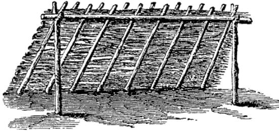
for flooring above the snow or damp. A common plan is to support a cross-bar by two uprights, as shown in the figure; against this cross-bar a number of poles are made to lean; on the back of the poles abundance of fir branches are laid horizontally; and lastly, on the back of these are another set of leaning poles, in order to secure them by their weight.
