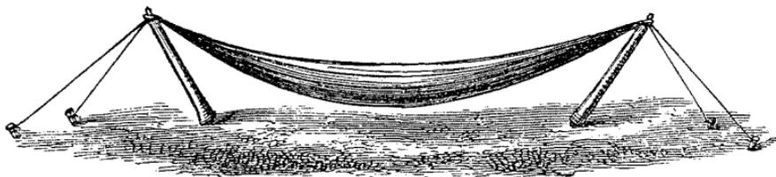
ratus is adapted for use on the wooden floors of houses or ships, by the employment of eyelet-bolts or screw rings instead of pegs, and by putting wooden shoes below the staves
