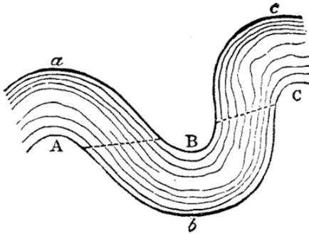
straight across, but follows the direction of a line connecting a promontory on one side to the nearest promontory on the other, as in the drawing; that is to say, from A to B, or from B to c, and *not* right across from B to *b*, from A to *a*, or from c to *c*. Along hollow
