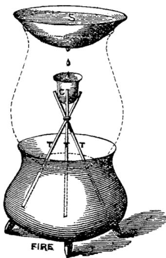
collected in a cup, c, that is supported by a rude tripod of sticks, t, standing in the inside of the iron pot.
