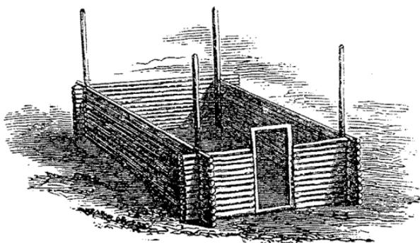
spaces between the logs must be caulked with moss, &c., or the log-cabin will be little better than a log-cage. It requires a great many logs to make a hut; for, supposing the walls to be 8 feet high, and the trees to average 8 inches in diameter,
