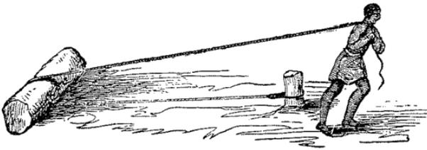
cases a more practicable one, is to make fast one end of the rope to the log itself; then, winding the rope two or three times round it, like cotton on a reel, to haul at the free end as before. Horses can be used, as well as men, for this work.
