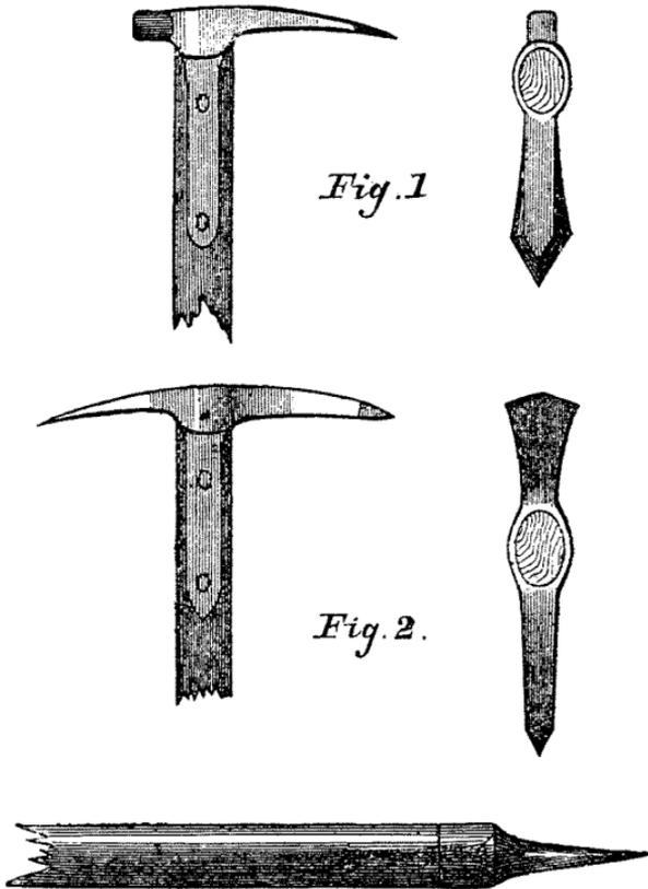
In the first place it is absolutely necessary that one of the cutters should be made in the form of a pick, as this is by far the best instrument for hacking into hard ice, and is also extremely convenient for holding on to a snow-slope, or hooking into crannies, or on to ledges of rock.
