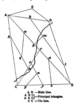
and commanding a good view; let the points be near the boundaries of the ground, and so situated that the line joining them forms a sort of diagonal; this becomes the main line.
