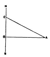
known, whence that of a neighbouring peak or land-mark, C, is to be determined; the distance AC must be measured, and the azimuth NCA observed, then the difference of longitude AB is the sine of ACB to radius AC, and the difference of latitude BC is the co-sine to the same angle and radius.
