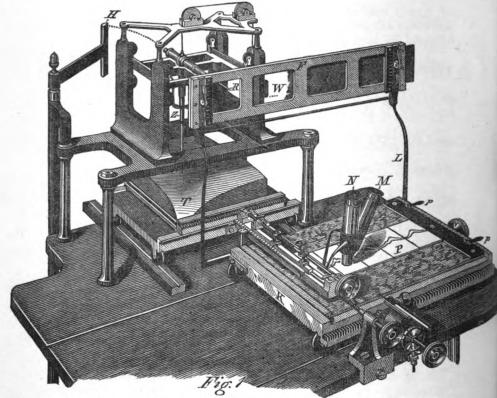
The machine consists of three portions. The first portion comprises a carriage K, shewn only in Fig. 1, which moves on tramways, from side to side. Its motion is governed by turning the lowermost of the three milled heads shewn at the bottom of the drawing, the axis of this milled head carrying a pinion in gear with rack work fixed to the carriage. On the same axis
