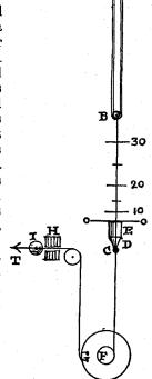
the top of E is brought level with the zero line. There C stops, owing to I coming in contact with the buffers H. Consequently the ivory cylinder E is tossed up as a free projectile, and the graduation to which it ascends is noted. The number attached to that graduation shows the number of feet per second at which T was moving immediately before its motion was checked.
